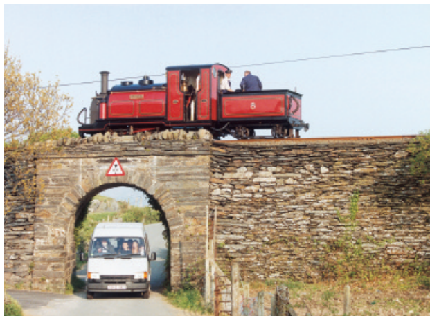
Awaiting his turn on Gwyndy Bank on 2 May 1999 is Prince, as a van demonstrates that the loading gauge for bridges over lanes is as confined as that for locos working on the FR.
